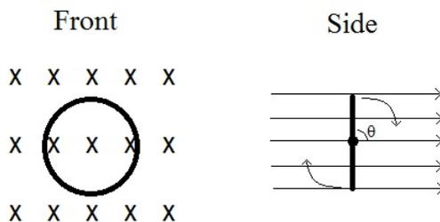
**Problem 4** The solenoid below has a radius of 2.0 cm, 10 loops/cm. A loop of resistance  $R = 2\ \Omega$  is placed around the solenoid with a radius of 5.0 cm. The current through the solenoid is given by  $i(t) = 5t^2 - 3$  A.
